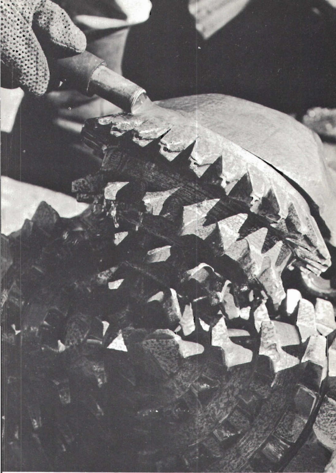
Greasing a 36 inch rock bit before spudding in an offshore well in Bass Strait.
